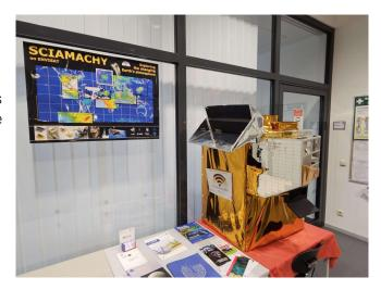
SCanning Imaging Absorption spectroMeter for Atmospheric CartograpHY (SCIAMACHY) designed in IUP was an imaging spectrometer on board the European Space Agency's (ESA) ENVISAT mission that provided unique global observations of pollutants including Greenhouse Gases and aerosols in the atmosphere from 2002-2012.
